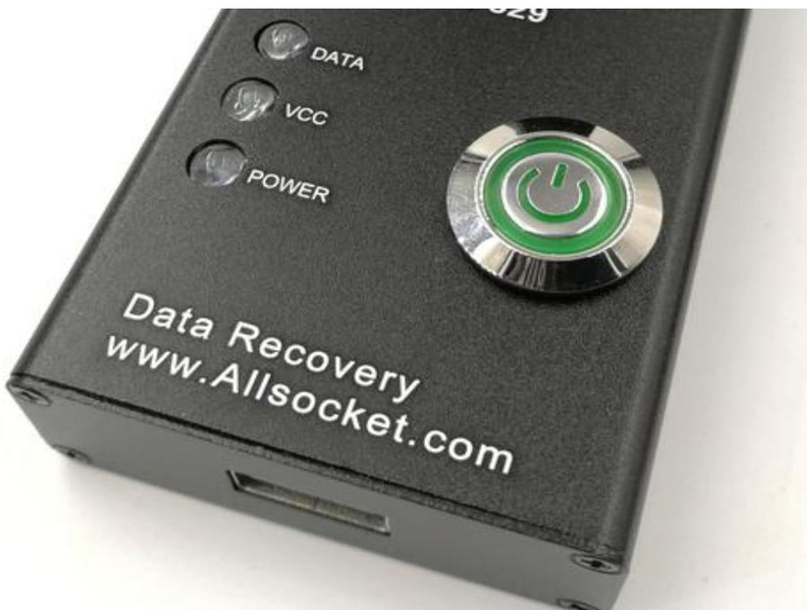
a). The LED at DATA is flashing at the beginning when start to read data, and then the light keep steady, the same goes with the VCC and POWER.
