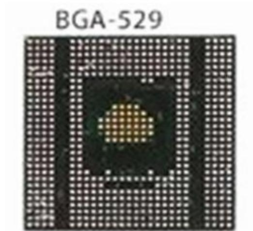
Galaxy Note4 use Multi-chip Memory chipset. There are two layers on BGA529 chip, the bottom part is what the Memory chip is.
